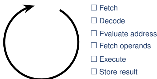
Figure 1.1: The instruction processing cycle (von Neumann model): six conceptual phases, repeated for every instruction.
